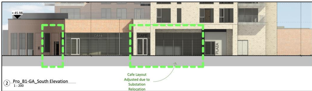
Figure 4. Extract from Drawing ‘Block 01 – Elevations – Proposed’ Drawing No. ‘19016A-OMP-B1-ZZ-DR-A-2101’, showing the proposed relocation of the substation and meter room adjoining the café unit, prepared by O’Mahony Pike Architects.
