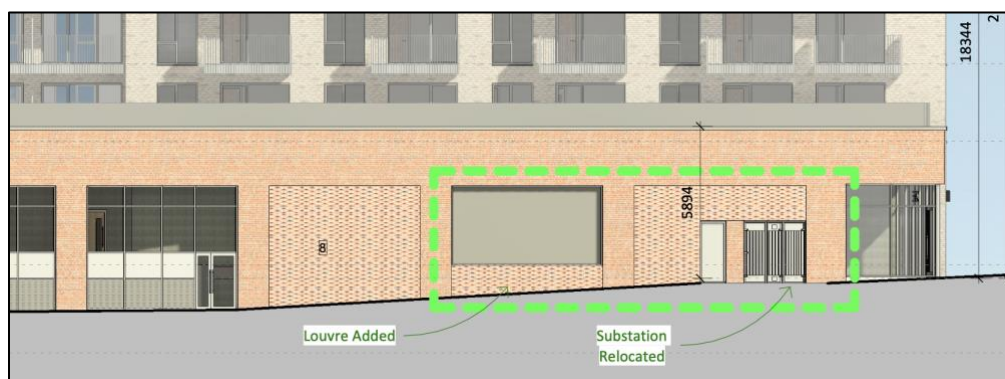
Figure 6. Extract from Drawing 'Block 01 – Elevations – Proposed' Drawing No. '19016A-OMP-B1-ZZ-DR-A-2101', showing the proposed relocation of the substation and meter room adjoining the café unit, prepared by O'Mahony Pike Architects.
