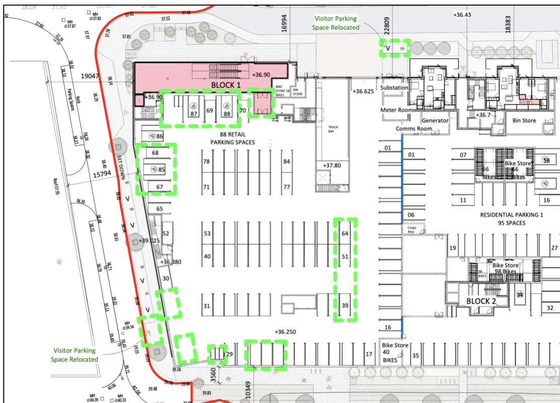
Figure 1. Extract from the Drawing ‘Site Plan – Undercroft Level 0 - Proposed’, Drawing No. ‘19016A-OMP-ZZ-ST-DR-A-1101’.
